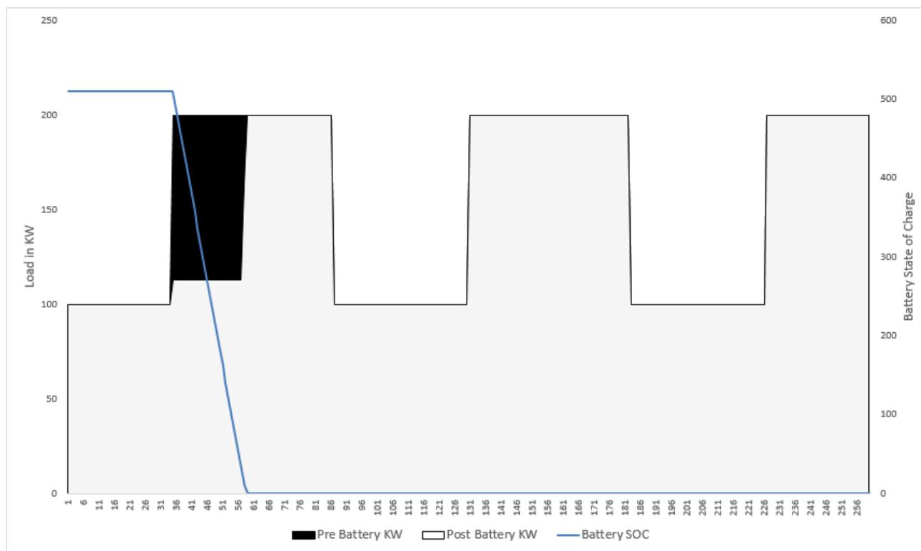
Figure 5: Illustration of battery operations for a typical “block” load profile (sample 360 “15 min” intervals): GI Energy
