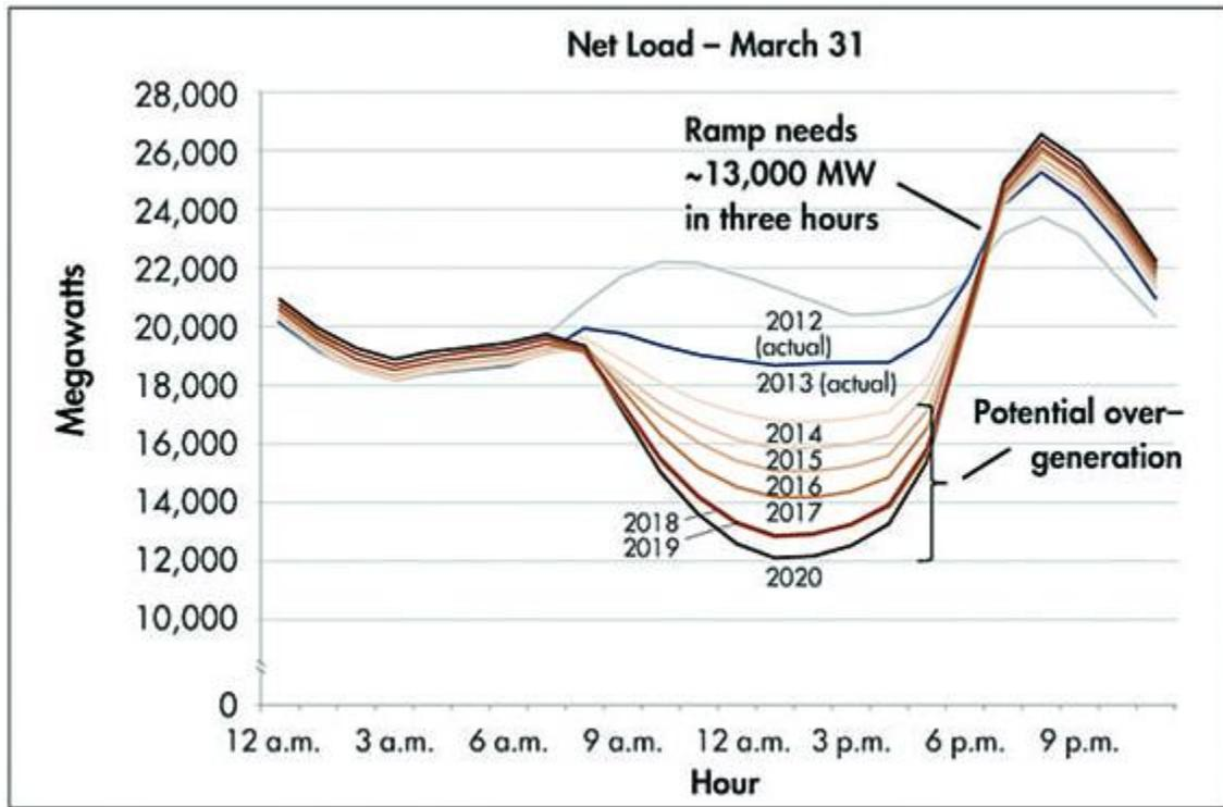
Figure 1: Illustration of the “duck curve” in California: Source CAISO
