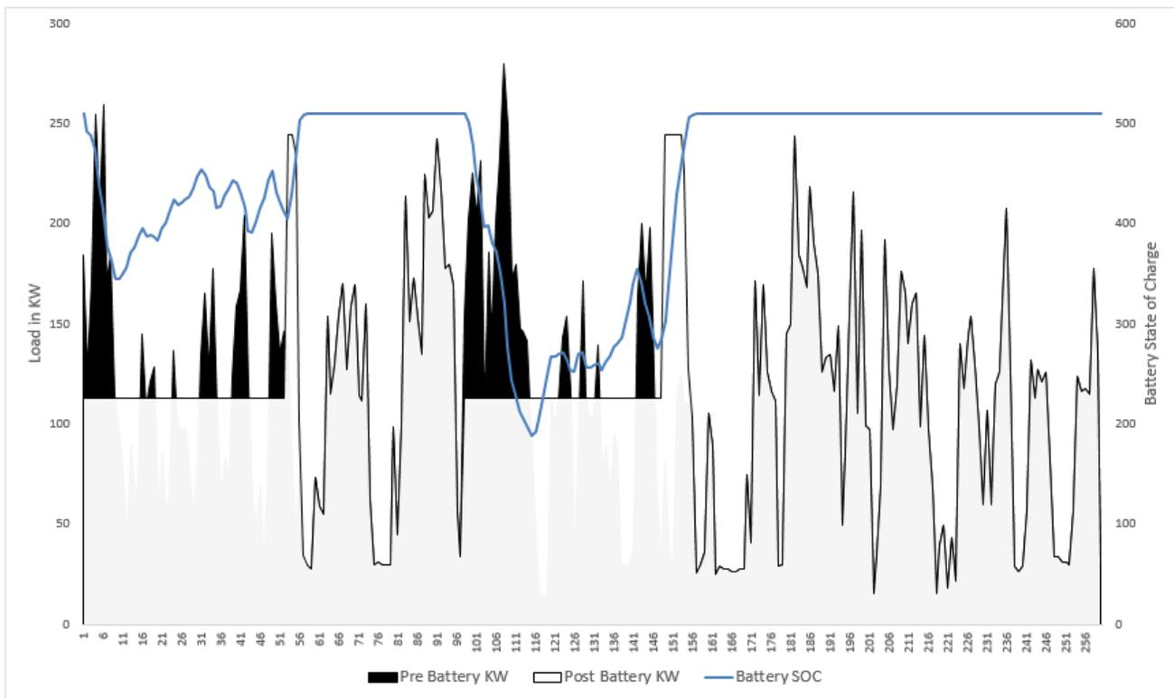
Figure 4: Illustration of battery operations for a typical “peaky” load profile (sample 360 “15 min” intervals) : GI Energy
